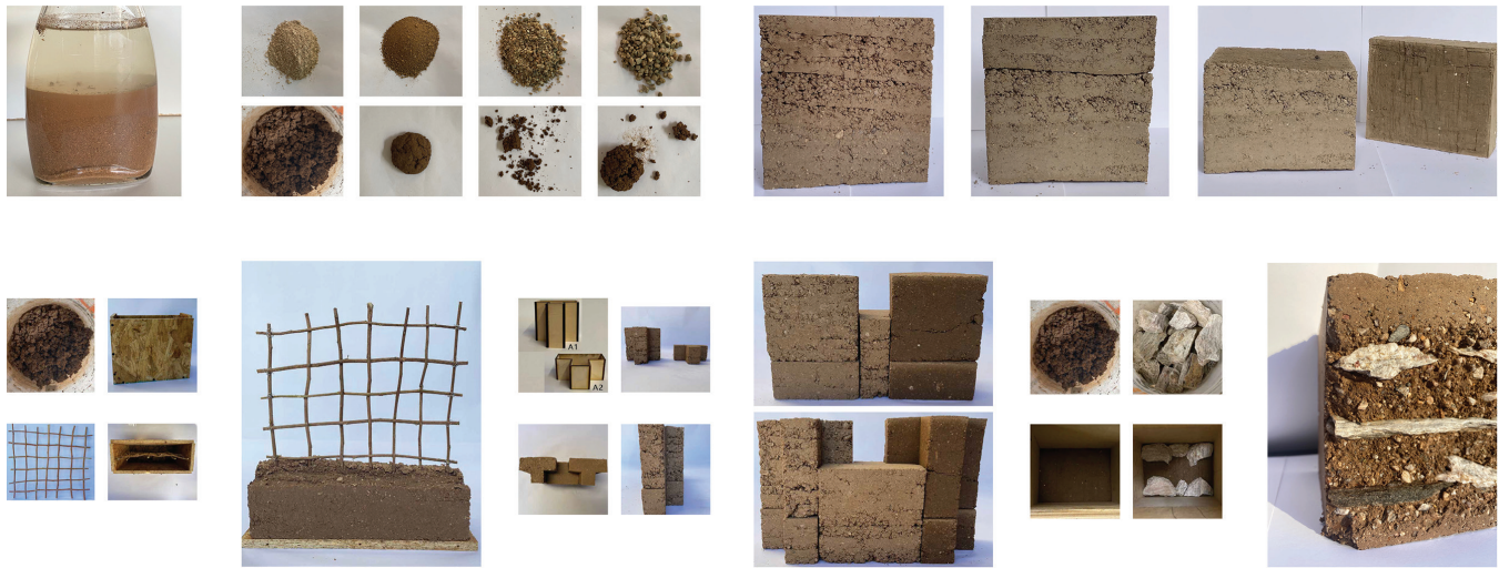
Figure 1. Initial studies with earth. Top row: exploring mixes, stabilized vs. unstabilized rammed earth, lower row: exploring various tectonic logics and details (Aracely Cervantes 2022).
